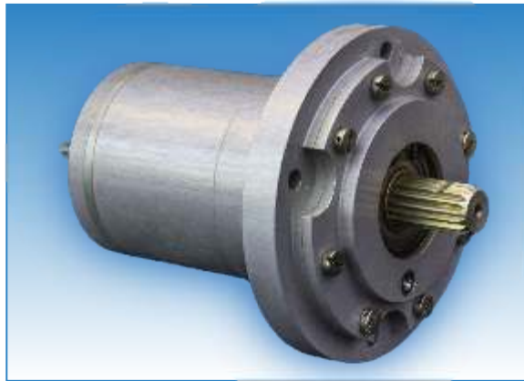
Aerospace elevator G-weight control damper. 120° travel vane type with integral temperature compensation.
